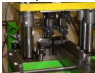
Nut piercing unit integrated into the production line
