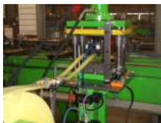
Feeding of the piercing nuts from refillable magazines
