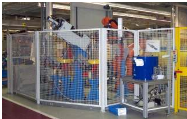
Piercing nut processing in assembly area with robot handling
