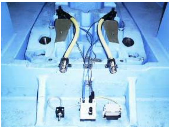
Piercing nut system, integrated into press tooling
